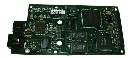
The PEP (Programmable Ethernet Port) board is a proven low-risk approach for new and existing power amplifier vendors and has already been qualified as being compliant with General Dynamics specifications for timing, frequency hopping, and proprietary Ethernet message protocol.
